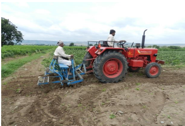
Sowing with seed drill
