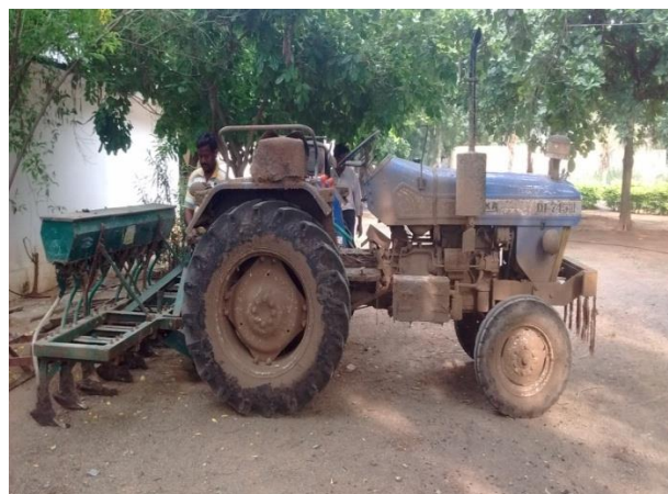
Sowing with seed drill
