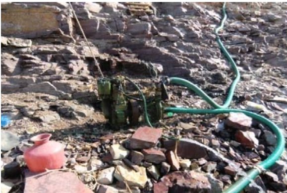
Oil Engine for lifting Irrigation water
